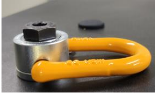
Pic.1 install eye-bolt
